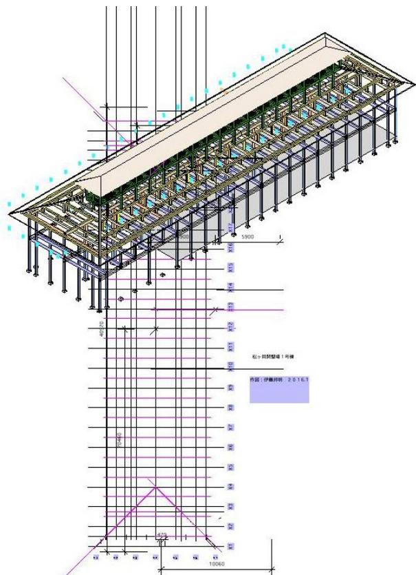
Fig.4. Structural system of No.1 silkworm house
